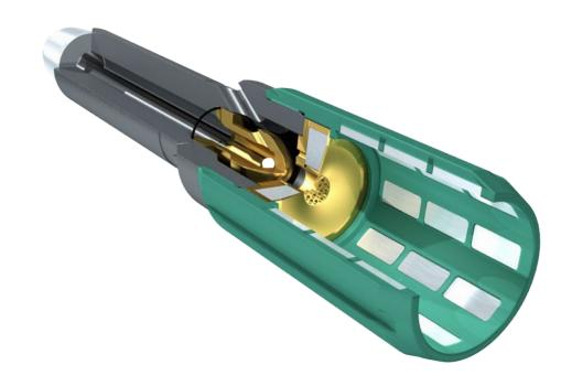
The MAGVac Fishing Magnet is a robust magnetic junk retrieval tool with reverse circulating technology that sucks junk into a magnetic overshot for safe retrieval to surface.
