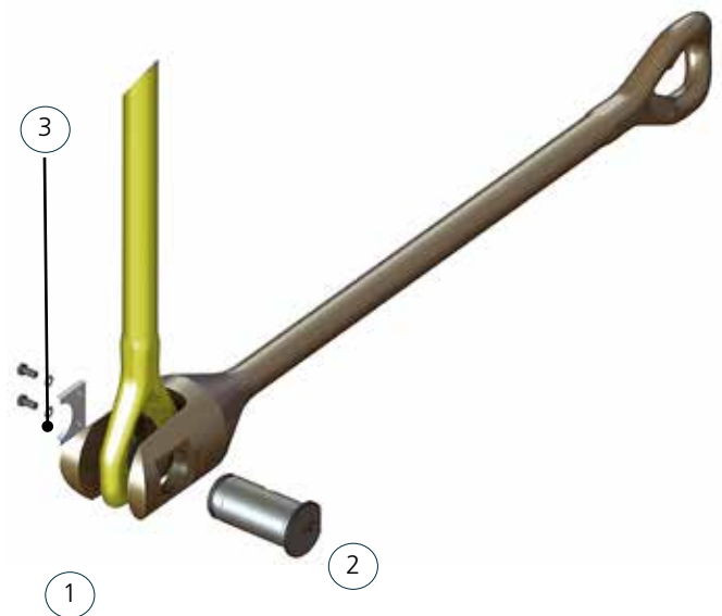
Fig. 11: Mounting the Elevator Link Extension to the Elevator Links
