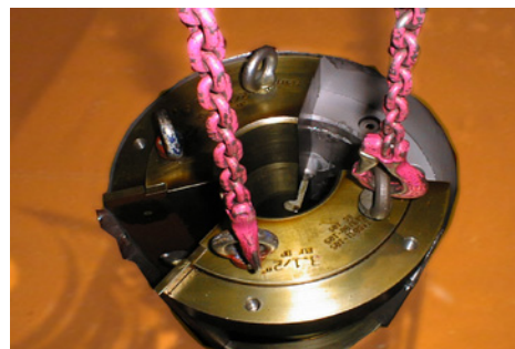
Fig. 33: Remove bushing VES SDS
