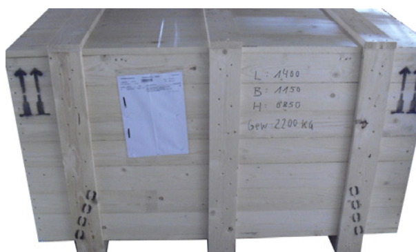
Fig. 29: Typical transport and conservation packing for SDS
