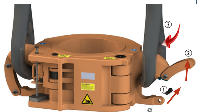
Fig. 36: Mounting the SDS to elevator links
