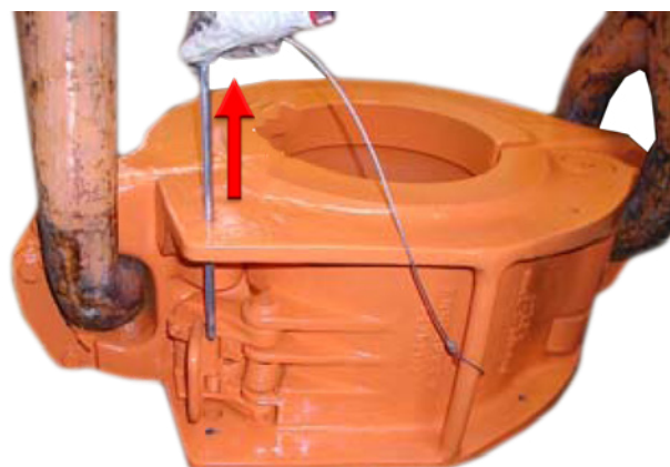
Fig. 39: Verification Pin operation position
