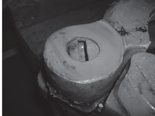
Figure 1: Lock bar removed correctly
