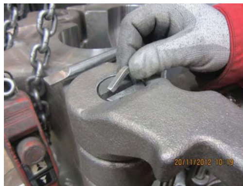
Placing the lockbar/hinge or latch pin retainer
