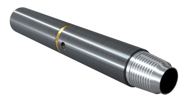
The **Rupture Disc Sub** is a tool activated by applying pressure from surface to burst a rupture disc to allow communication between the workstring and the annulus at a predetermined pressure. The tool has two calibrated rupture discs to provide redundancy.
