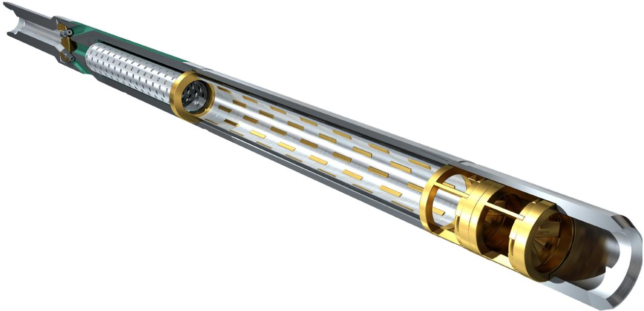
The **ARdVAC™ Venturi XTRactR™ Tool** is a robust, Venturi type debris extraction tool which vacuums debris and junk from the wellbore. It can be deployed in most common casing or hole sizes and can be adapted to clean inside packer bores. It can be run individually or modularly as part of the ArmRdillo™ Wellbore Clean-Up System.
