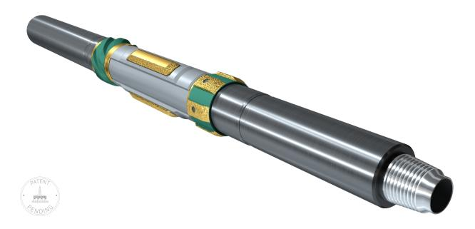
The MillRdillo Deburring Tool™ is a robust milling tool designed to safely mill hard inclusions on the on the casing inner diameter without causing damage. It can be run individually or modularly as part of the ArmRdillo Wellbore Clean-Up System.
