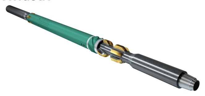
The PiRanha™ Junk XTractR™ is a robust, free-rotating wellbore clean-up tool and can be run individually or modularly as part of the ArmRdillo™ Wellbore Clean-Up System. The PiRanha™ Junk XTractR™ is designed to mill up and remove junk from the wellbore which could damage downhole equipment.
