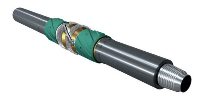
The ScourRdillo™ Casing Brush is a robust, 360° contact, free-rotating wellbore clean-up tool and can be run individually or modularly as part of the ArmRdillo™ Wellbore Clean-Up System. The ScourRdillo™ Casing Brush can be adapted to suit any casing size and drill pipe combination.
