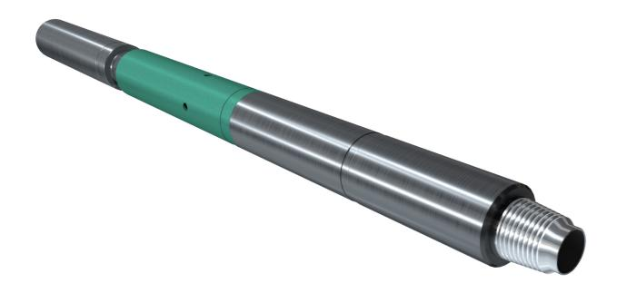
The Weight Set Circulating Tool is a robust and simple circulating tool which can be opened and closed by string manipulation. It is typically run above a Liner Top to allow circulation of the casing above the liner. The Weight Set Circulating Tool is available to suit common casing and liner combinations.
