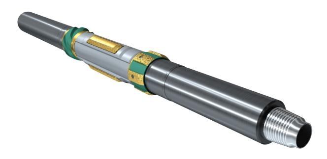
The MillRdillo Deburring Tool™ is a robust milling tool designed to safely mill hard inclusions on the on the casing inner diameter without causing damage. It can be run individually or modularly as part of the ArmRdillo Wellbore Clean-Up System.
