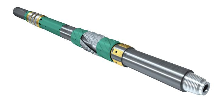
The DTectR™ Inflow Test Packer is a simple but effective well integrity testing device which performs a negative pressure test on a liner top. The design of the tool allows the test to be performed during wellbore cleaning operations, eliminating the need for a separate trip in hole.
