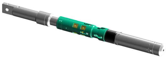
A hydraulically retrievable packer designed for use as either a temporary or permanent barrier. It allows for the application of maximum loads, torque, and tension throughout the setting, milling, and retrieval processes.
