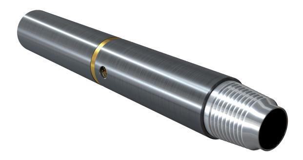
The Multi-Cycle Circulation Sub is a highly versatile and robust drilling valve specifically engineered for use in drilling operations and Wellbore Clean-Up Bottom Hole Assemblies (BHAs). It features a straightforward dart drop mechanism, which facilitates the repeated opening and closing of circulation ports. This valve may be utilized independently or as a modular component within the ArmRdillo™ Wellbore Clean-Up System..
