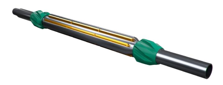
The UltraMag™ HD Casing Magnet is a highly robust, high-capacity casing magnet with free-rotating upper and lower centralisers. It can be run individually or modularly as part of the OTL Wellbore Clean-Up System and can suit any casing size and drill pipe combination.
