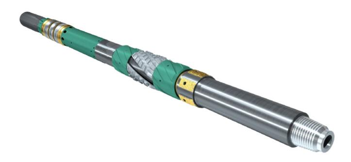
The DTectR™ Inflow Test Packer is a simple but effective well integrity testing device which performs a negative pressure test on a liner top. The design of the tool allows the test to be performed during wellbore cleaning operations, eliminating the need for a separate trip in hole.
