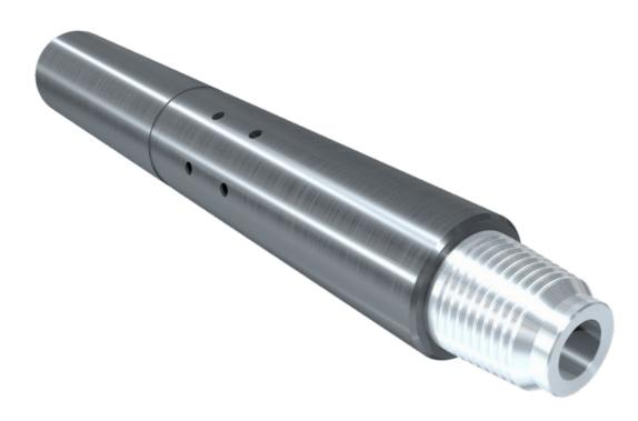
The Emergency By-Pass Sub is a robust and simple circulation tool that allows communication path from the drillstring to the annulus. Typically run as part of an ArmRdilloTM Wellbore Clean-Up System it is placed above filtration tools as an emergency bypass in the event of the filter tool plugging.
