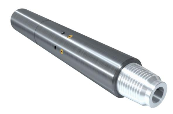
The Packer Circulating Tool is run with open circulation ports to allow circulation above a packer and to auto-fill the string whilst RIH. When desired the ports can be closed to allow setting of the packer.
